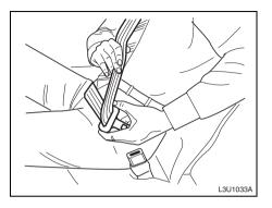
Pull up on the latch plate to make sure it is secure.
